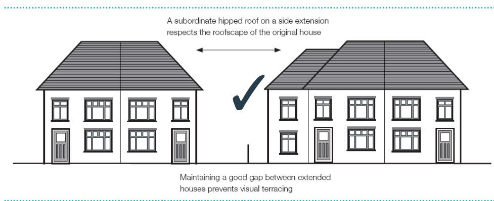
Figure 3: Maintain gaps between houses with subordinate extensions
